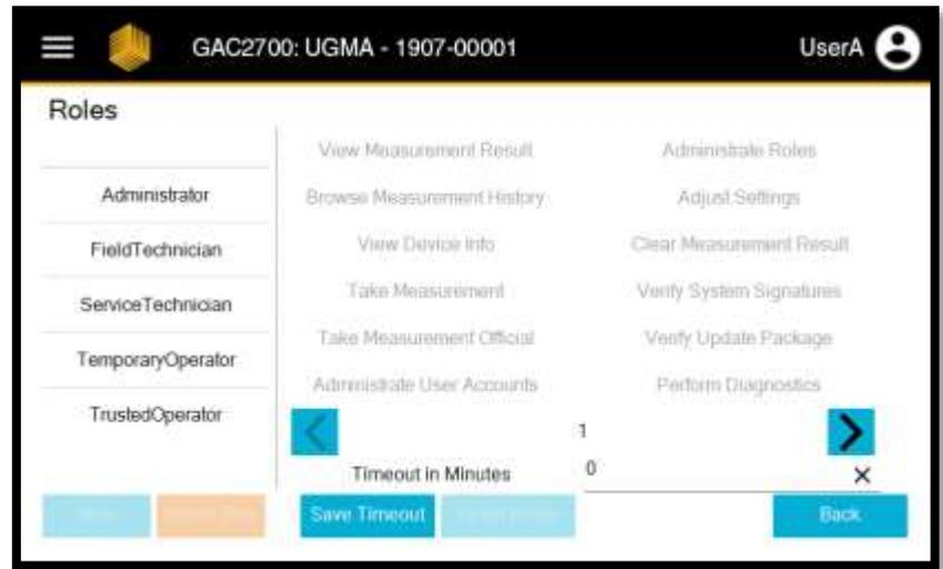
The GAC® 2700 can create preset lists of permissions which are called 'Roles'. These sets of permissions will allow the admin to define whether a specific operator is able to only conduct a moisture measurement, adjust settings, download new software, all of these, none of these, or conduct other interactions with the GAC® 2700.
