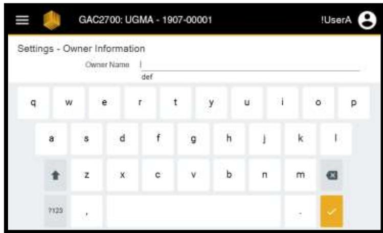
The GAC® 2700 permits the user to apply owner information into the instrument memory in order to aid with asset tracking.
