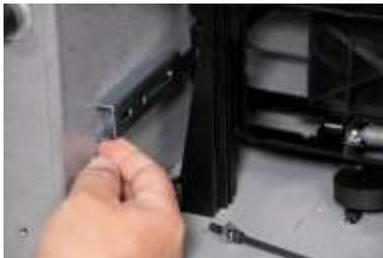
8. Insert the hex bolt into the operating location hold and tighten using the Allen wrench.
