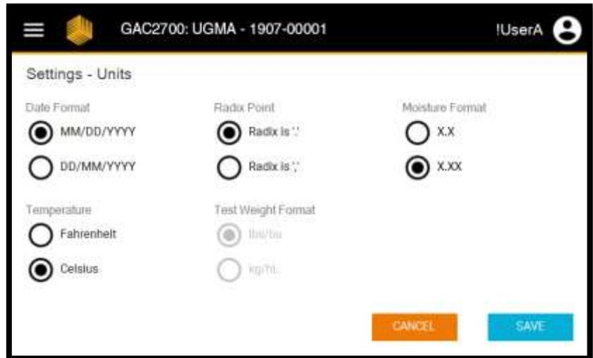
The GAC® 2700 is capable of delivering results in both imperial and metric units in order to meet the needs of the global grain moisture measurement market. For some areas of the world, these settings will be automatically set by the Region setting. For all others, the operator is able to make these changes in this menu screen. Settings in black font can be modified while setting in gray font cannot be modified.
