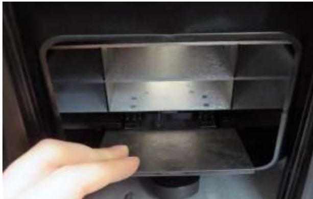
7. Clean surfaces around measurement cell including hinge, trap door, and edge of cell with the supplied brush.
