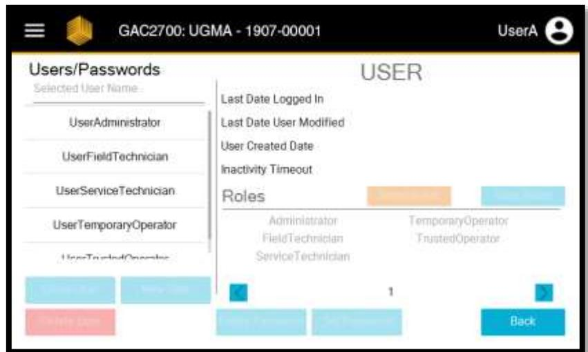
The GAC® 2700 can be configured for multiple levels of user interaction with the settings that would affect metrology of the instrument. This menu provides the Admin with the ability to configure what pre-defined set of permissions a user would have in the form of roles.
