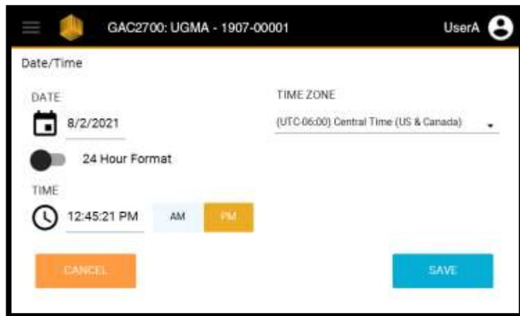
Throughout the course of the instrument life, it may be necessary to adjust the date or the time on the GAC<sup>®</sup> 2700 so that the measurement is accurately recorded. This screen allows the authorized user to change the date and/or time.
