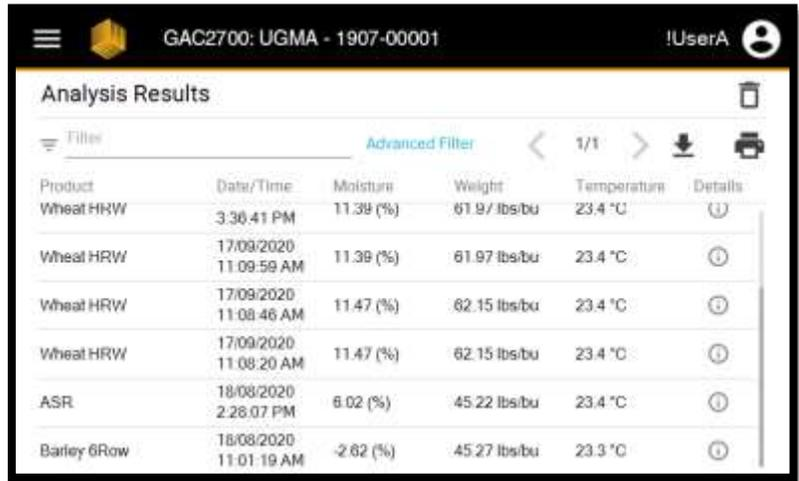
The GAC® 2700 is equipped with memory to store approximately 3,000 moisture measurement results consisting of all parameters of the measurement. Items such as the grain name, moisture and test weight results, the temperature of the grain at time of measurement, user ID, sample, ID, etc. are all available on this screen.
