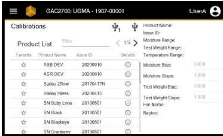
The GAC® 2700 is shipped with product calibrations that are tied to specific regions of the world. Once a specific region has been selected during the initial set-up, the GAC® 2700 automatically displays the relevant group of calibrations tied to that region. In many instances, this list includes both Official and Unofficial calibrations:
