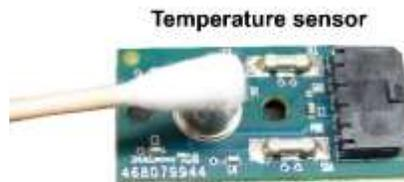
5. Allow the temperature sensor to dry for 90 seconds then gently clean with the dry end of the cotton swab.
